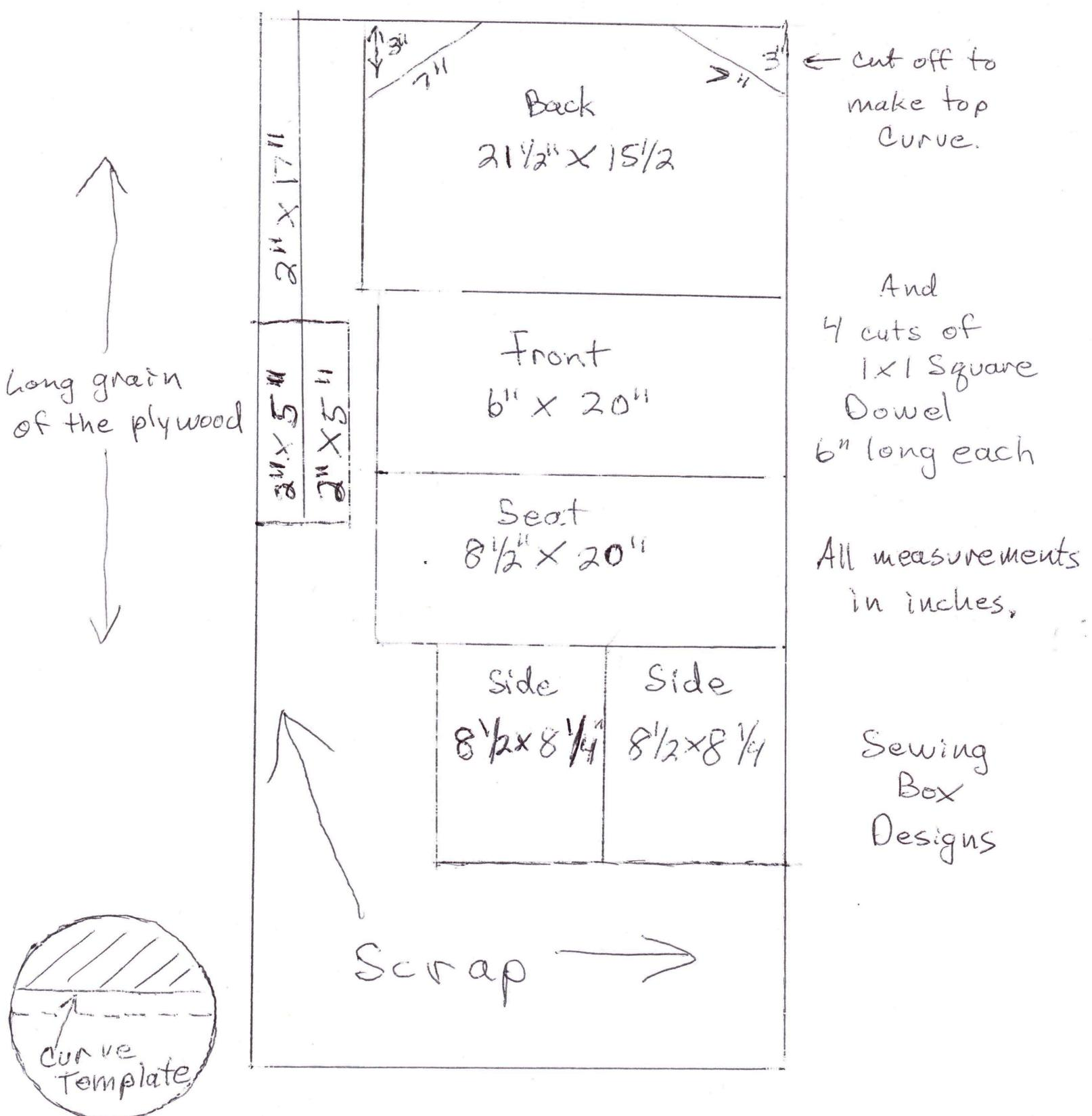
To make the templates for the curved cut outs, make a 6" and 8" diameter circle. Fold in half, then mark 1 inch up. Center the smaller template on side, the larger is for the back and front.
